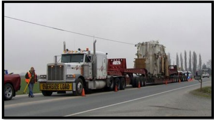
Example of a super-load that requires bridge loading analysis.
